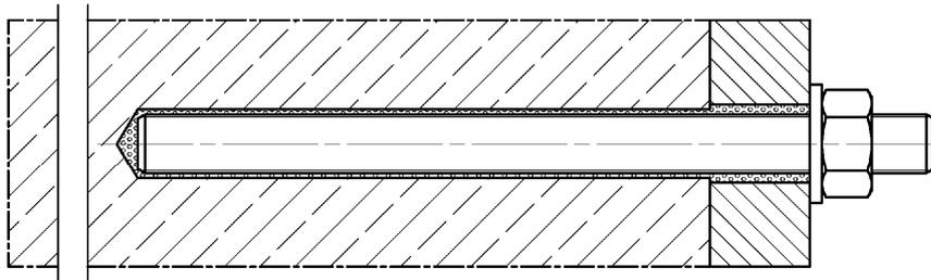
**Pre-positioned or push through installation with subsequently injected fischer filling disc**
