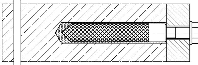
Pre-positioned installation with subsequently injected fischer filling disc (annular gap filled with mortar)
