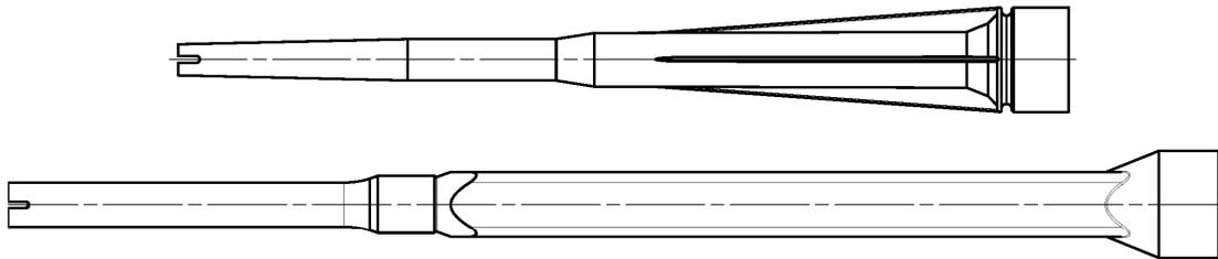
**Injection adapter / extension tube for static mixer**
